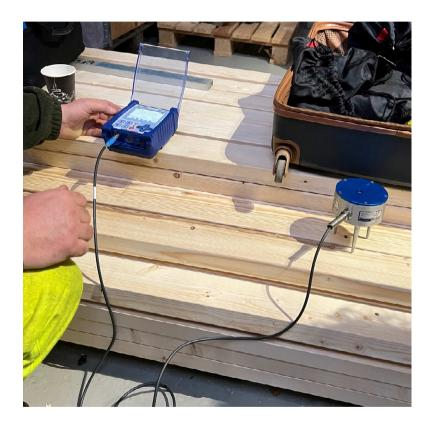
Sensitive measuring equipment ensures that the vibrations do not exceed the limit value
